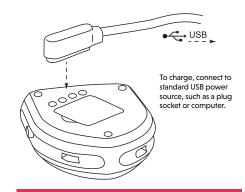
**DO NOT OVERCHARGE** - 2 hours should be quite sufficient and longer charges tend to degrade battery life and performance.
