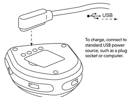
**DO NOT OVERCHARGE** - 2 hours should be quite sufficient and longer charges tend to degrade battery life and performance.
